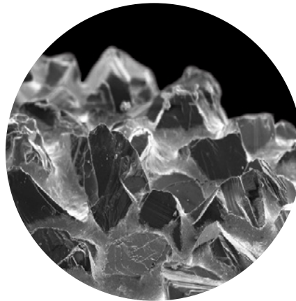
High magnification photo of diamond crystals on a Two Striper® instrument.
