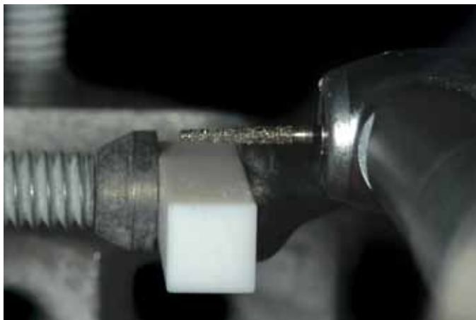
1 Bur cutting surface shown paralleling material.
