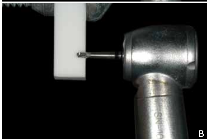
2 A, Alignment of bur 1 mm from edge of substrate. B, Alignment of carbide burs with short cutting surface lengths on block.
